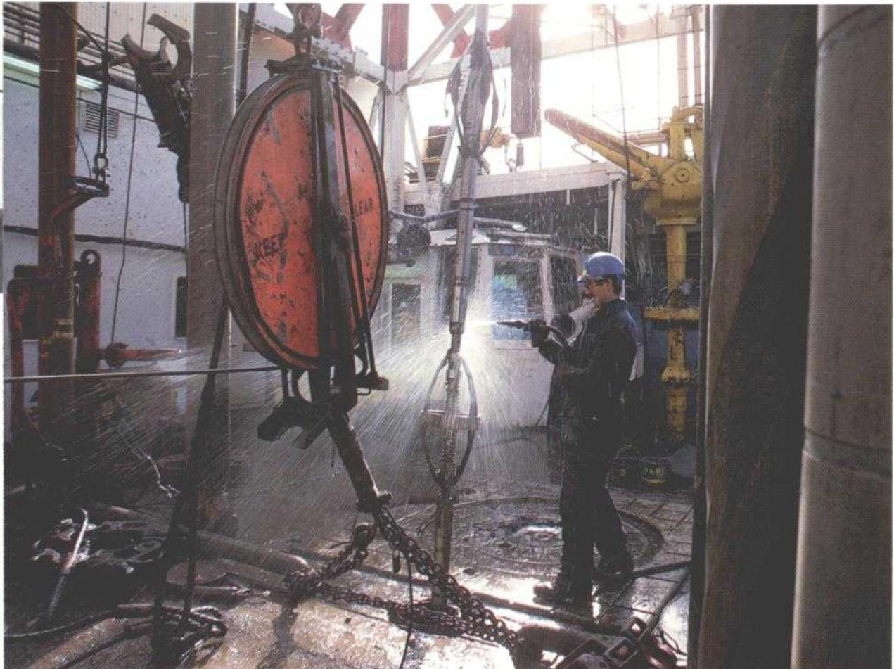
*Technician washes well logging probe that has just been removed from well or "hole." On the floor to his right is the rotary table, which imparts rotary motion to the whole drill assembly. Well logging is an electronic technique to determine the potential of the drill location.*
