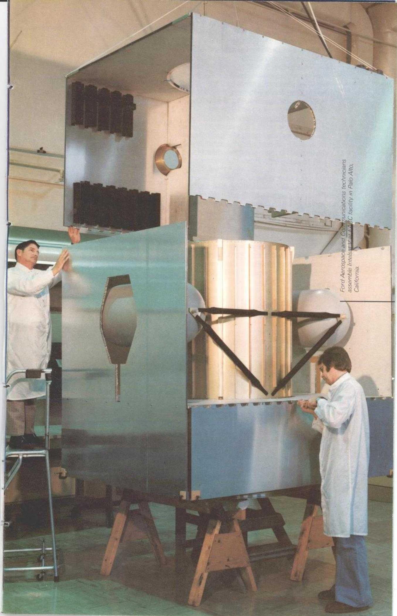
*Ford Aerospace and Communications technicians assemble Intelsat V at EAGC facility in Palo Alto, California.*
